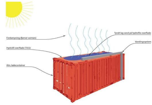
giving the roofs of the containers a coat of titanium dioxide (TiO<sub>2</sub>). When the water evaporates, according to thermodynamic principles it draws energy, i.e. heat, out of surface, thus cooling the container.
